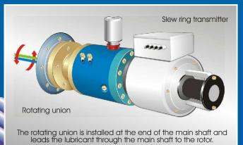
The whole lubricant supply is located in the nacelle.
