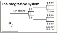
The progressive system supplies many lubrication points with just one feed line. It can be monitored easily and offers flexible extension possibilities. BEKA produces progressive systems from simple manifolds at the safety fence up to fully automatic systems.
