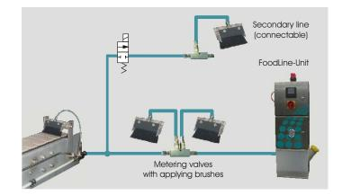
Working and break times of the system can be adjusted with the electronic control. Together with external signals, different lubrication cycles can be controlled.
