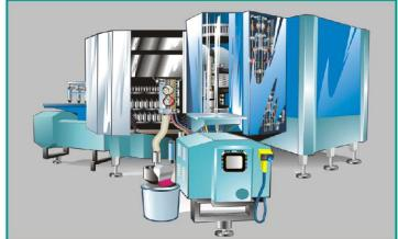
Automatic FoodLine maintenance systems supply all machines in the filling and packaging industry with lubricant.
