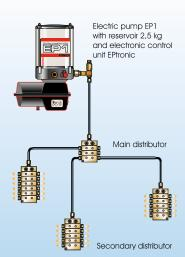
The electronic control of the central lubrication is adapted to the operating conditions of the vehicle and activates the pump in defined intervals.
